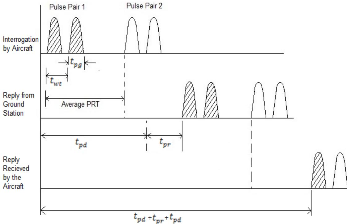
Figure 1: DME Pulse Waveform
