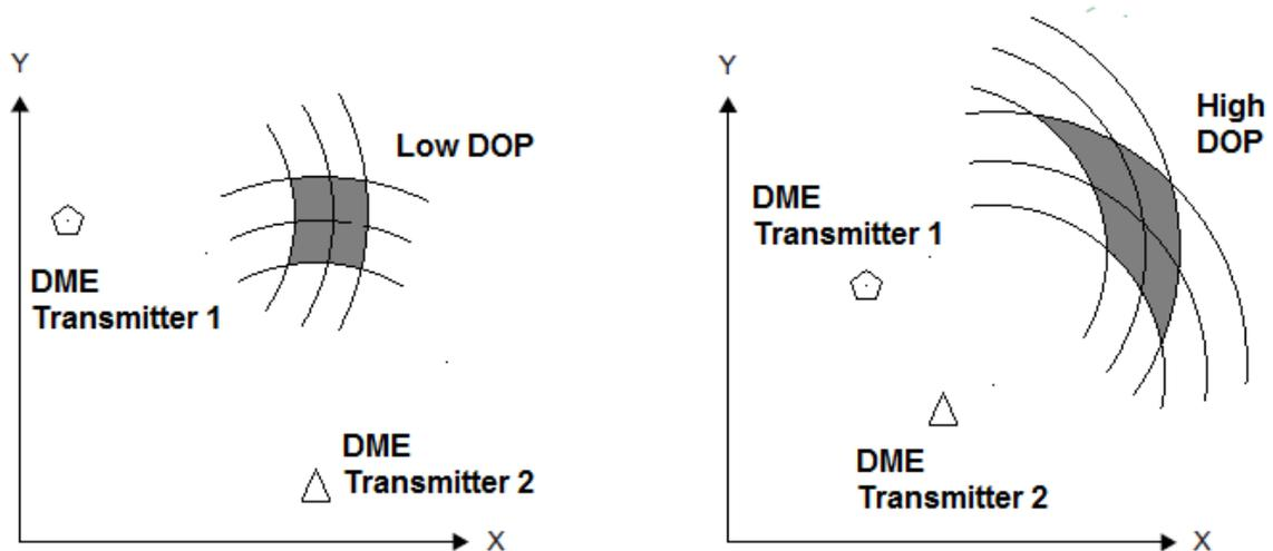
**Figure 2: Uncertainty of Receiver's Position Depending on Transmitter's Geometry**
