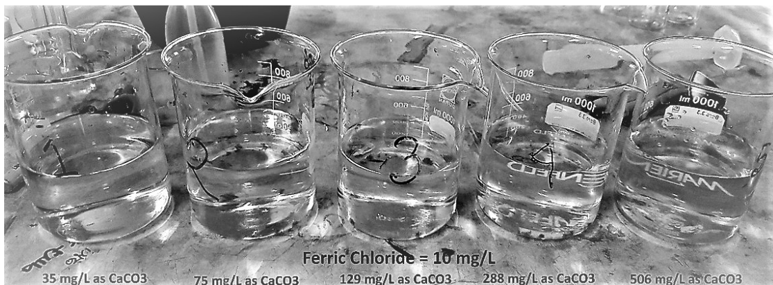
Figure 5: Effect of Alkalinity on Formation of Ferric Hydroxide Flocs during Coagulation with \text{FeCl}_3
