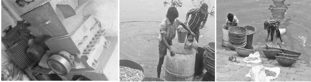
Figure 2: Shredding Machine (Left); Workers are Washing Shredded Plastic Pieces in Buriganga River (Right)
